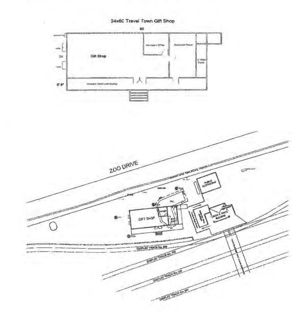
Below is the plan for the new building, as supplied by DSMB. Below that is a draft plan of the north side of Travel Town, with the new building outline in blue.
